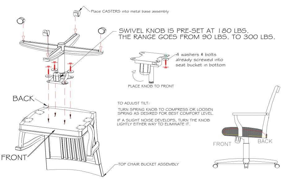
PRE-CAUTION: EVERY 6 MONTHS- RETIGHTEN THE 4 BOLTS IN THE MOUNTING PLATE. USAGE CAN MAKE SCREWS WORK LOOSE OVER TIME.
